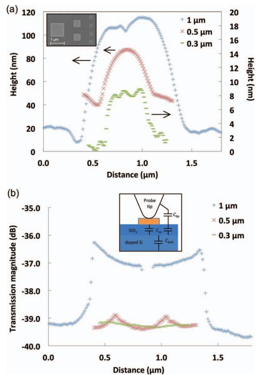
FIG. 5. (a) Profile of the AFM topography image of square capacitances with sides of 1, 0.5, and  $0.3 \mu\text{m}$ . The top left inset shows the top view of the capacitances obtained with scanning electron microscopy. (b) Profile of the transmission parameter magnitude measured across the center of the pads by the interferometer setup. The inset shows the parasitic capacitance  $C_{tip}$  coming from the probe tip over the  $\text{SiO}_2/\text{Si}$  substrate.
