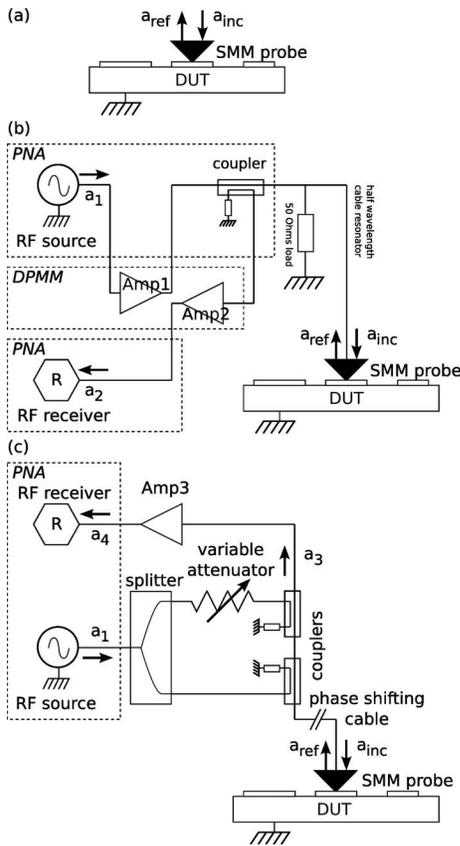
FIG. 1. (a) Definitions of the incident and reflected signal on the DUT. (b) Schematic of the Agilent Technologies SMM set-up integrating a 50  $\Omega$  resistor shunt and a half wavelength resonator in the probe holder. (c) Proposed set-up integrating an adjustable microwave interferometer based on a Mach-Zehnder configuration.
