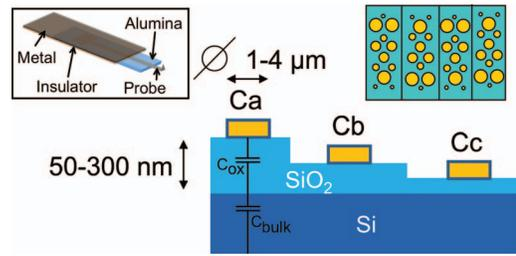
FIG. 3. Calibration kit based on scaled MOS capacitances. The  $\text{SiO}_2$  layer is etched to obtain steps with different thickness. The gold electrodes are deposited on the different  $\text{SiO}_2$  steps. The top right inset shows the top view of the calibration kit. The top left inset represents the AFM probe configuration with the ground plane (the view is upside down).
